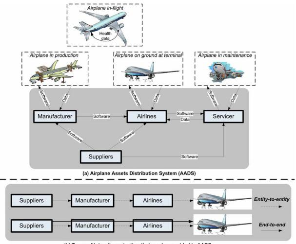
(b) Types of integrity protection that can be provided in AADS
