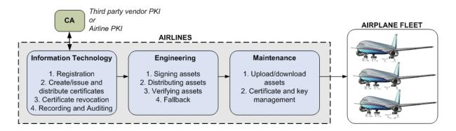
Fig. 2. An assignment of new operational requirements across typical departments at airlines
